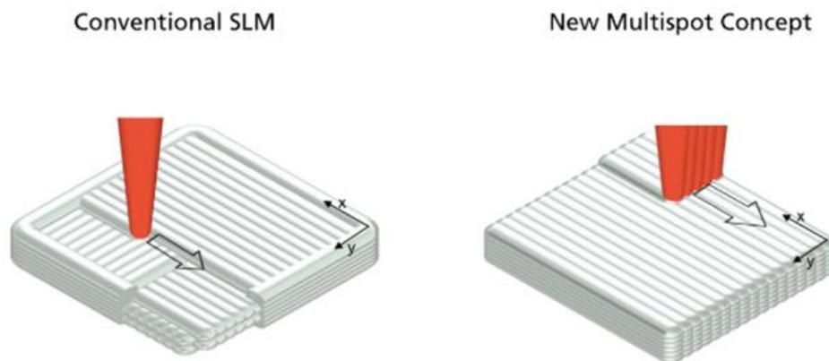
Figure 12. Comparison between conventional laser on SLM and multispot concept [50]
