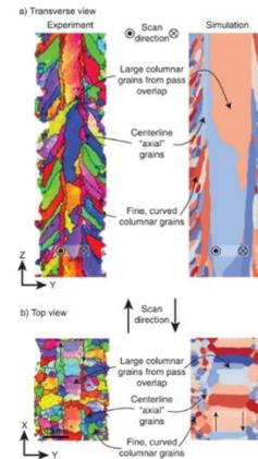
Figure 11. Comparison between experimental EBSD (left) and (right) simulated images.
