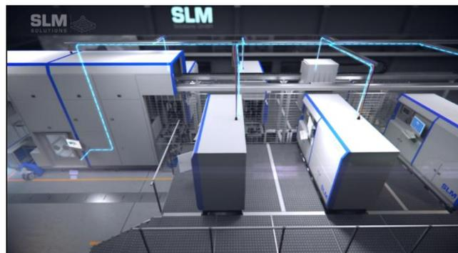
Figure 16. Automated powder transport (feed, extraction and recycling) from SLM Solutions
