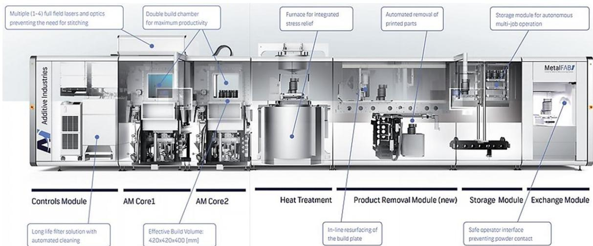
Figure 14. MetalFab1 system (Additive Industries) [52]
