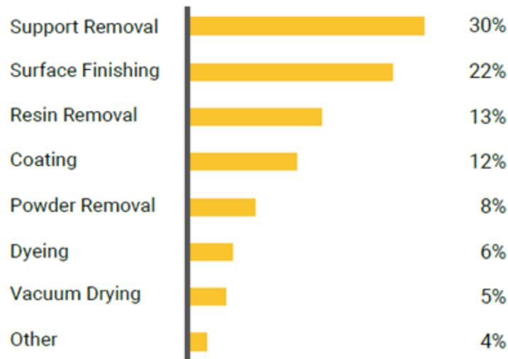
Figure 22. Top Post-processing. Source: Annual Additive Post-Printing Survey: Trends Report 2019. Post-Process
