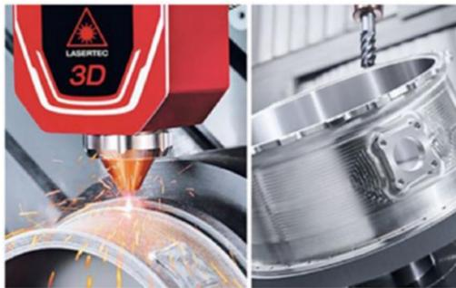
Figure 18. DMG MORI's hybrid process images
