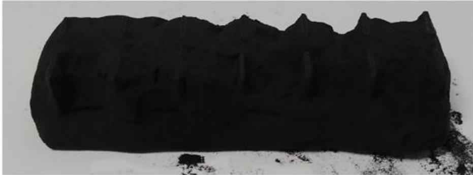
Figure 23: Example of an SLS part after the majority of bulk powder is removed
