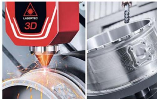
Figure 18. DMG MORI's hybrid process images
