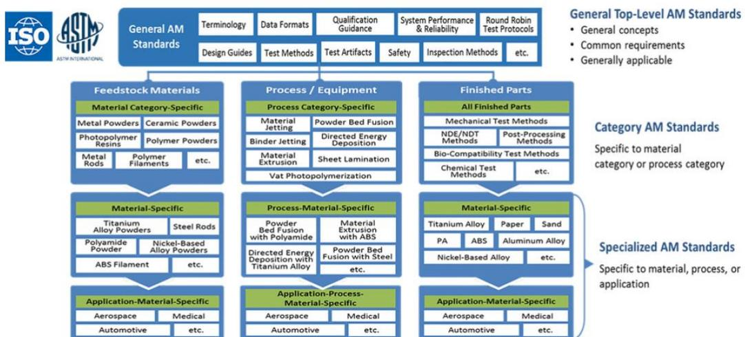
Figure 3 - Top level AM Standards defined by ISO and ASTM
