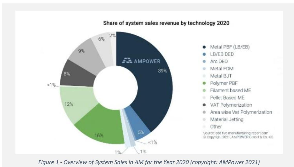
Figure 1 - Overview of System Sales in AM for the Year 2020 (copyright: AMPower 2021)
